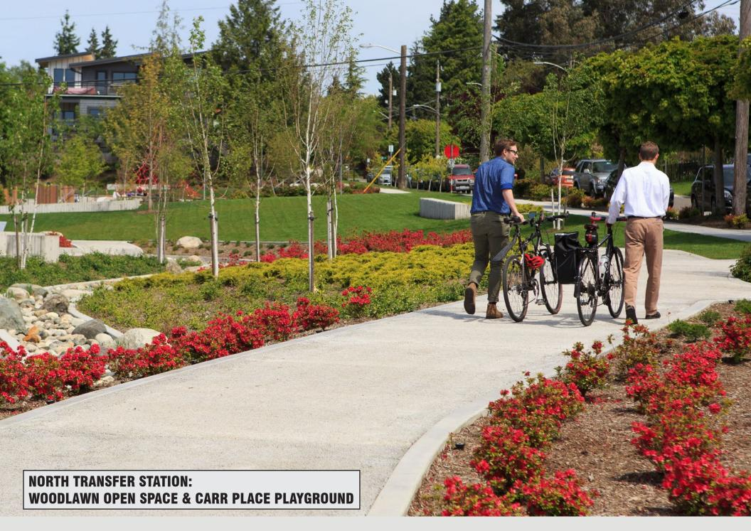
Generous pathway widths allow for comfortable walking and biking connectivity. The pathways are all permeable concrete.
