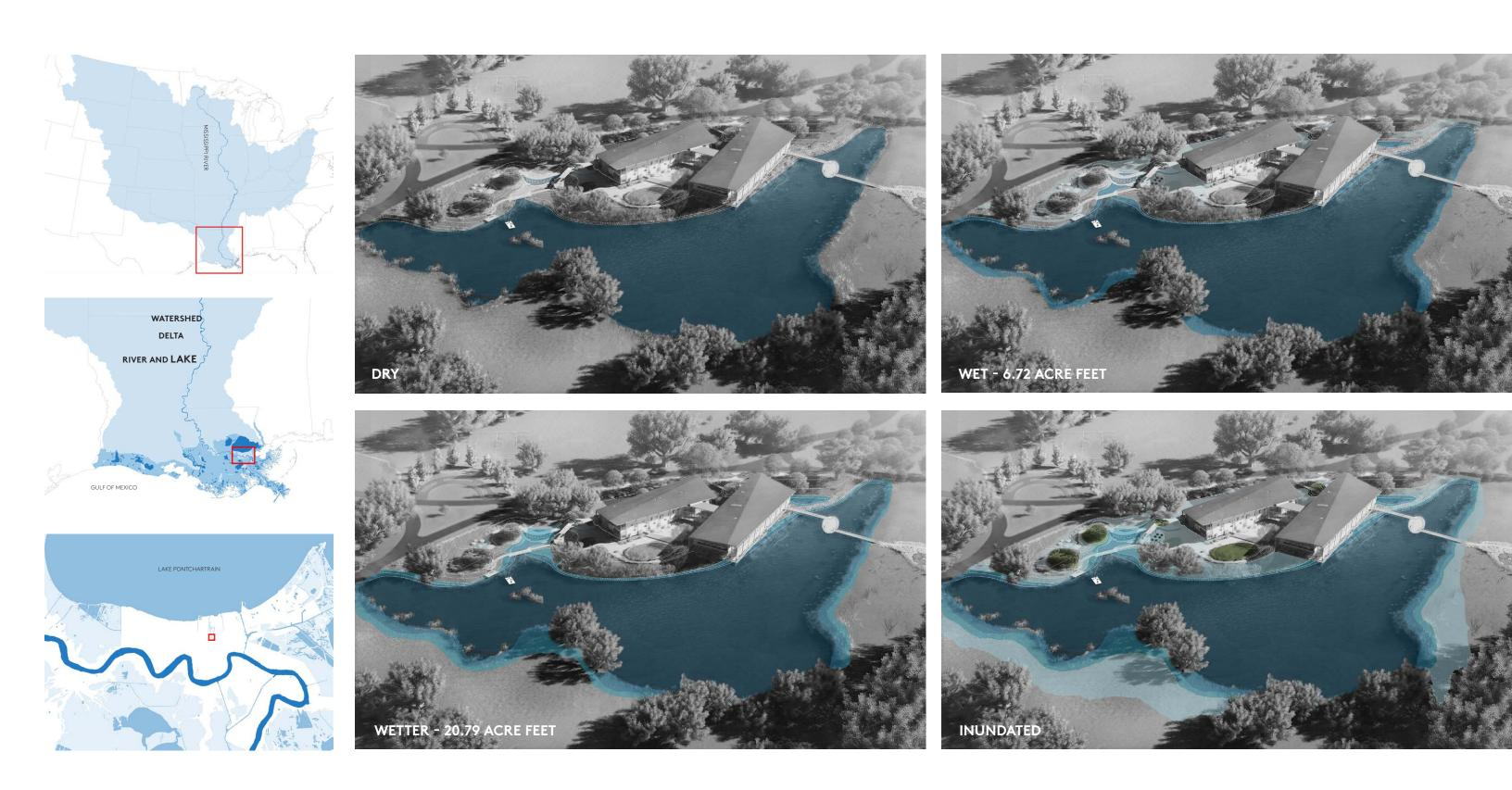
THE SITE IS DESIGNED TO STORE EVERYDAY FLOODING—UP TO THREE FEET OF WATER—AND IS AN EARLY DEMONSTRATION PROJECT OF THE GREATER NEW ORLEANS URBAN WATER PLAN. A SITES PILOT, THE PROJECT TARGETS LEED GOLD CERTIFICATION.
