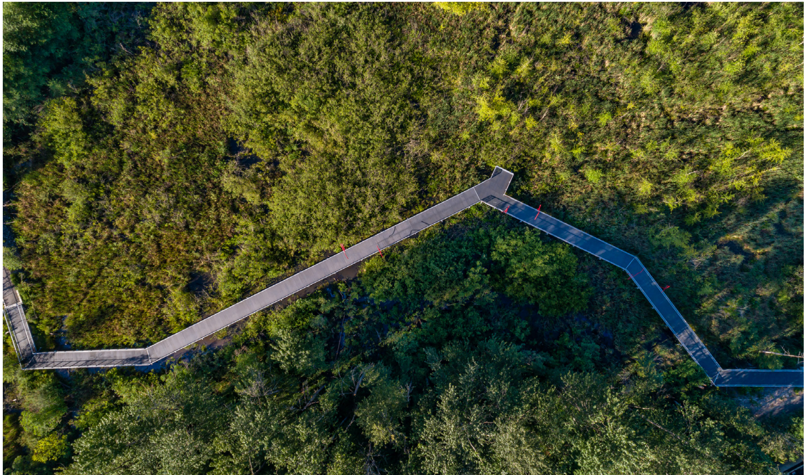
With the wetland inaccessible for survey or soils investigation, drone photography provided high quality imagery for the boardwalk design. Vegetation types were identified, and major trees mapped to avoid during construction. Invasive species were targeted for mitigation and restoration.
