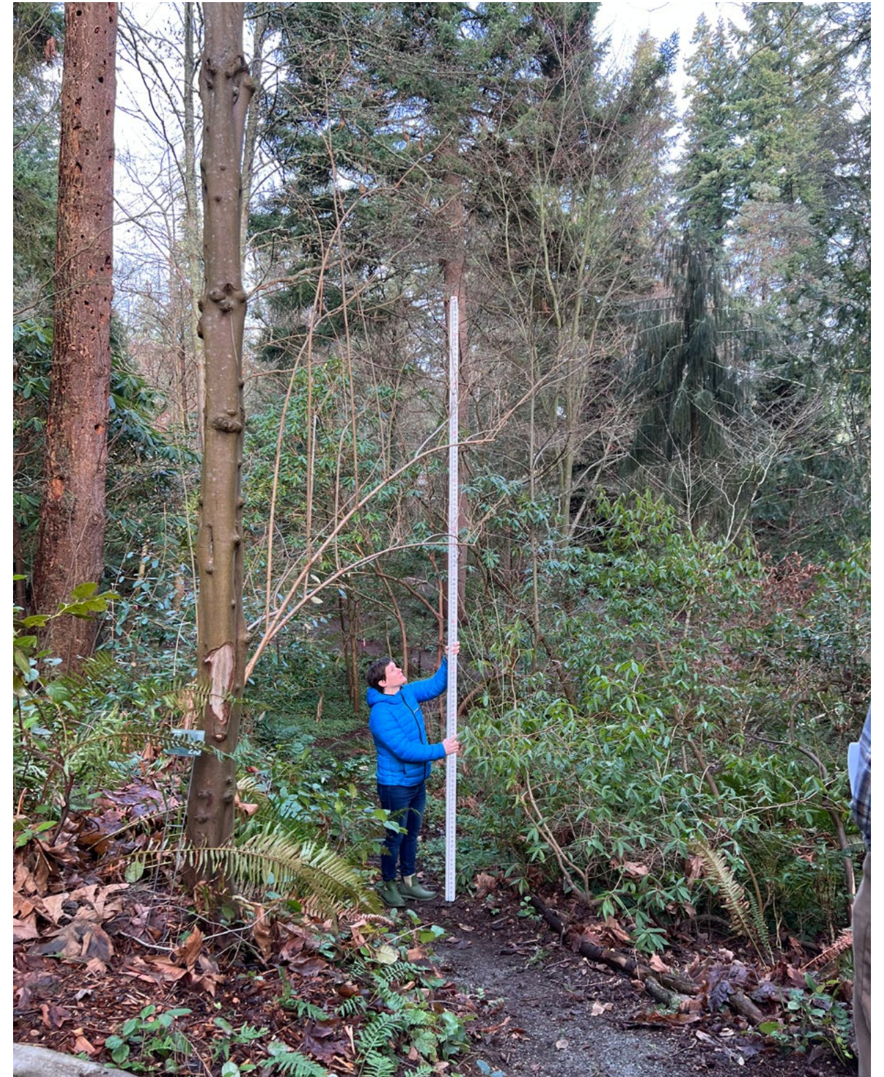
The design-build project team tested multiple layout options with survey poles, ladders and string to help the community visualize and understand the impacts of construction.
