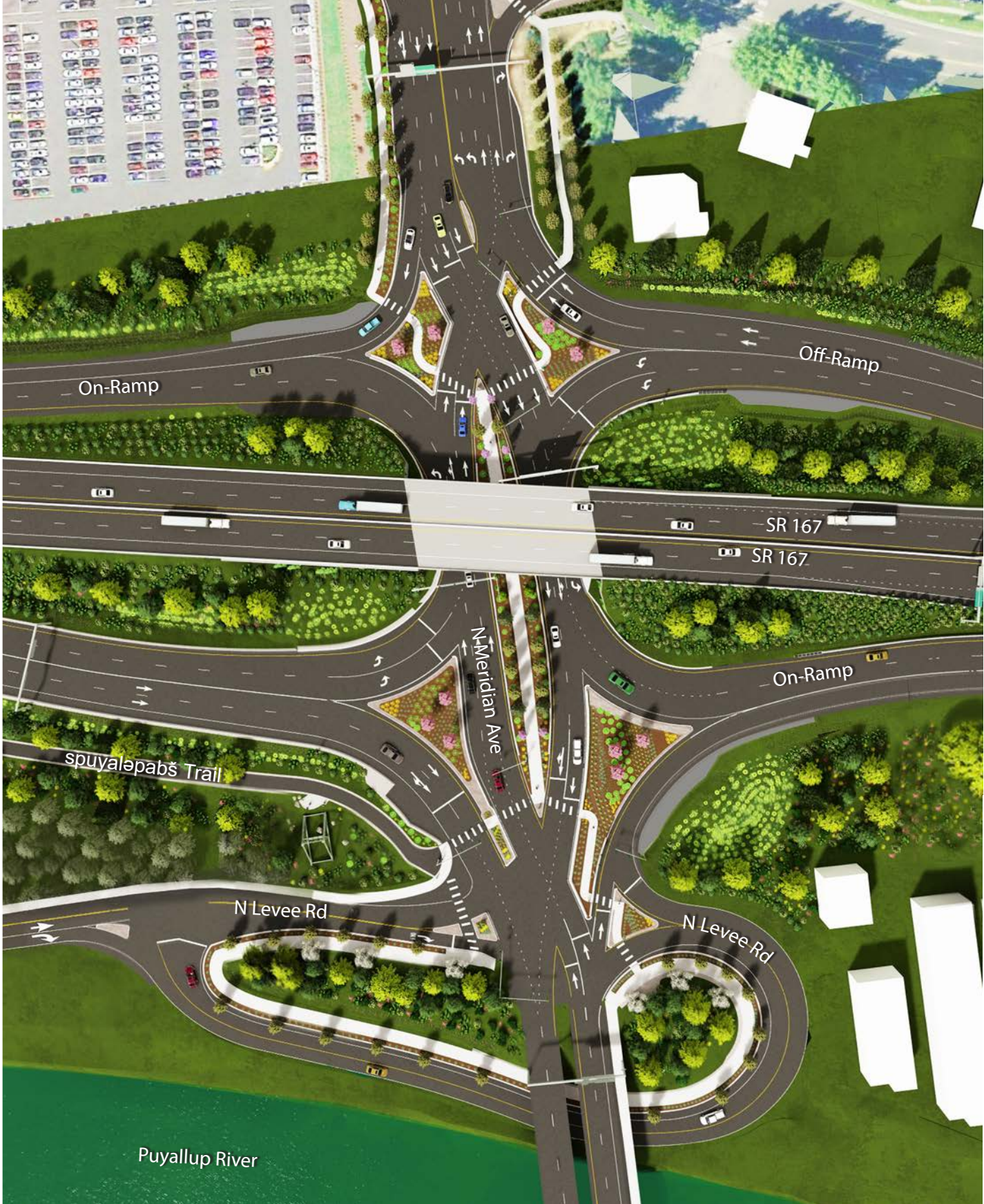
N MERIDIAN AVE INTERCHANGE | The Plan Map illustrating the diverging diamond interchange outlines the proposed treatments for roadside restoration. It addresses urban requirements, incorporates ecological enhancements, integrates historical elements, and responds to existing interfaces.
