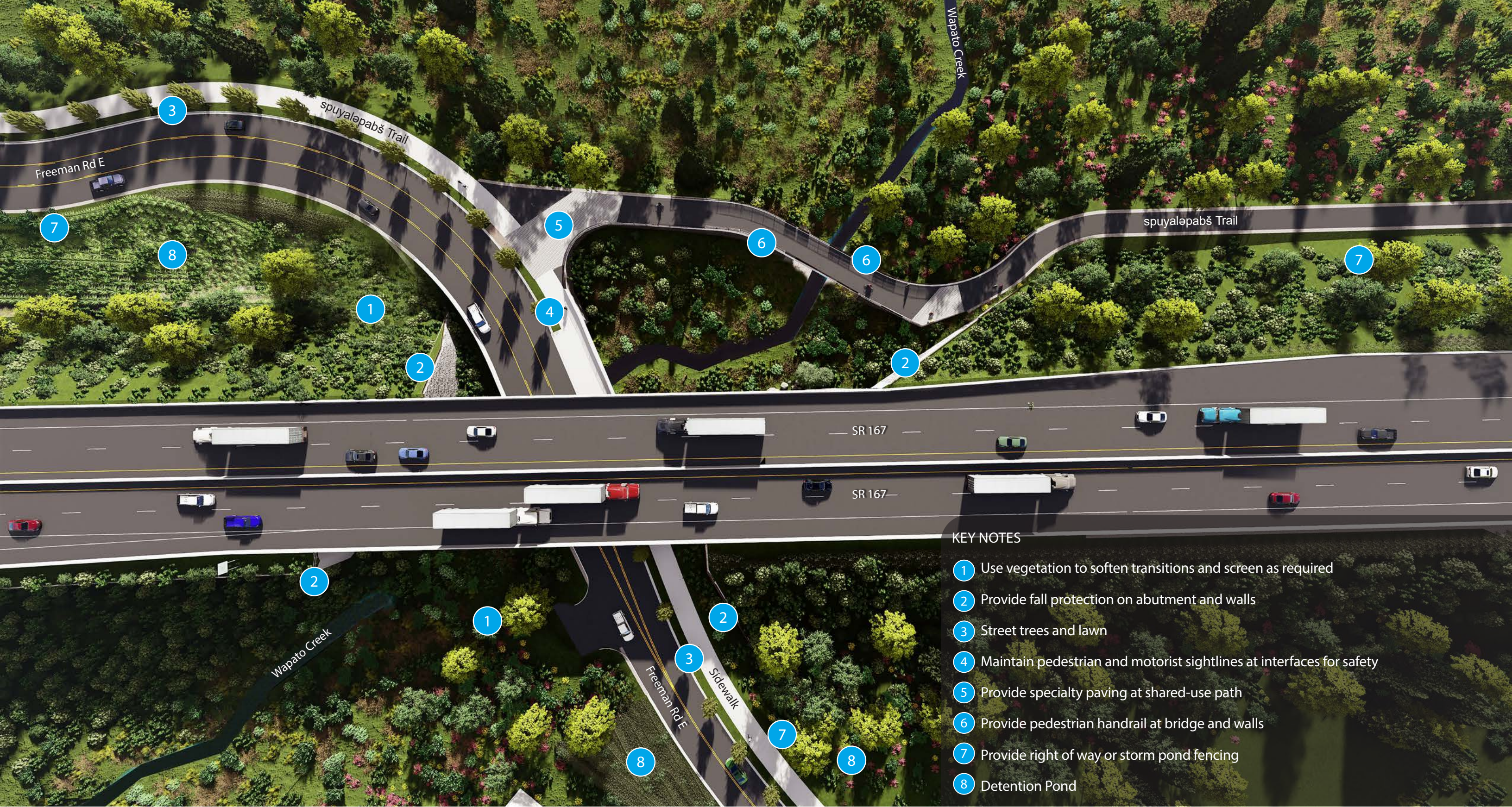
WAPTO CREEK AND FREEMAN ROAD OVERPASS | Plan rendering of the SR 167 overpass illustrating the connectivity between the spuyaləpabš Trail and city sidewalk interface and the preferred treatments for differing conditions.
