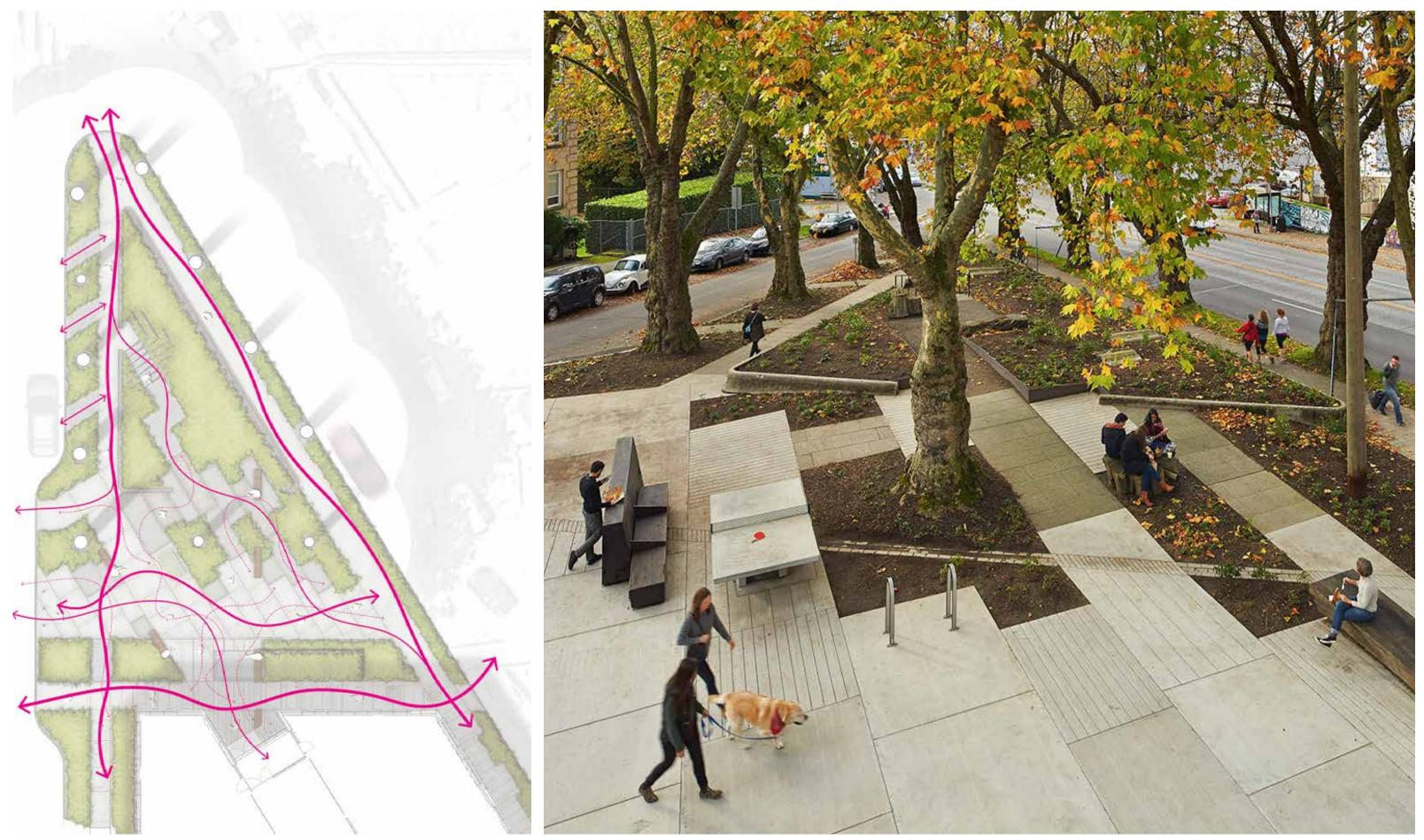
Curbless space is open to only non-motorized uses aside from emergency vehicles. New hardscape and grading required surgical insertion between existing trees. Every piece of existing hardscape in park was salvaged and reused onsite.
