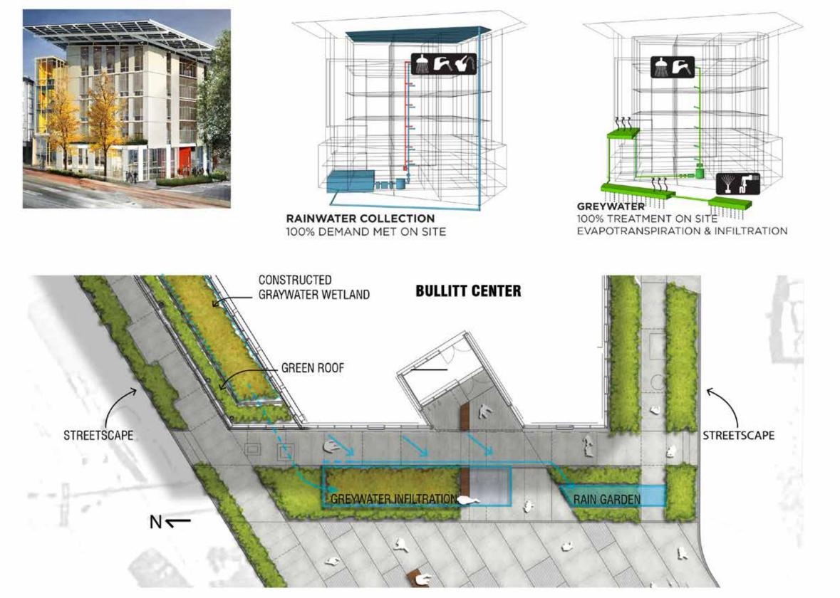
Rooftop rainwater is collected and used in the building for potable uses. Greywater flows to constructed wetlands to be treated and infiltrated through planters at grade. Stormwater flows to the rain garden. Permeable grating allows both function and access.
